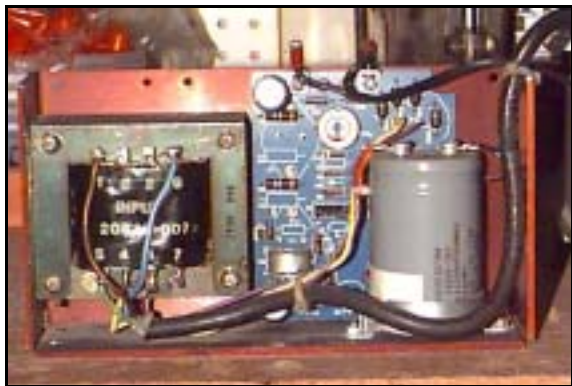
The charger I use is a 12 volt 6.5 amp power supply out of a scrapped industrial machine. The voltage adjustment potentiometer is between the transformer and the big filter capacitor.
