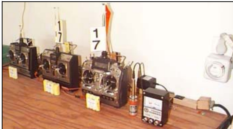
Above is my new charging station. The ESV on the right is used to periodically check the ready state of each pack. Right, on the wall, is the appliance timer, which powers the terminal strip (behind) that all the chargers are plugged into. It turns on for one hour each day and maintains all three flight packs and the glow starter at full charge. I have the timer set to come on at 6AM and go off at 7AM, so if I get up and decide to go fly, each pack has just been topped off and is good to go.
