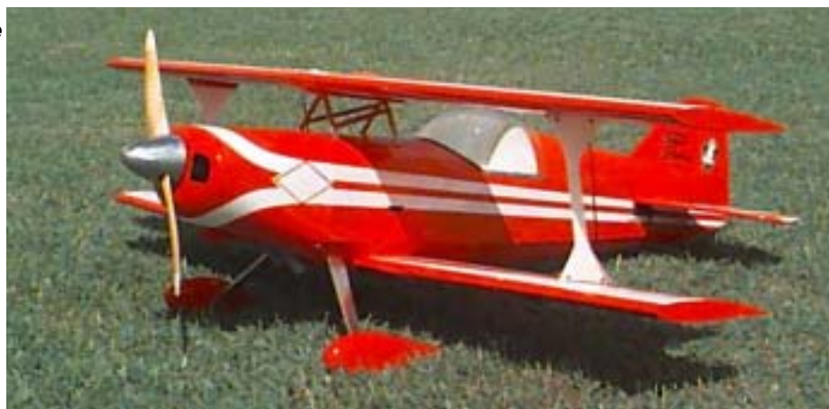
This little beauty is owned by Scott Driesse and on this day made it's maiden flight. It's a Midwest "Super Stinker" and is powered by a Moki 180. The ailerons and elevator both have duel servos. Bill Lancaster built the plane originally.
