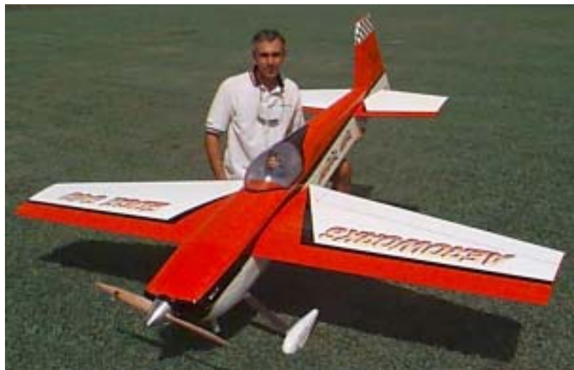
Here's Jerry Arcia's new 36% Edge 540 from Aero Works. It's powered by a 3W100SS, has all digital servos on the tail surfaces and JR 8101's through out the rest of the plane. Jerry used to have a 29% Edge and was really impressed with the way it flew, but he said this plane is so solid and stable that it's almost unbelievable. "Everything about the way this plane flies is much better than the 29%", Jerry said.
