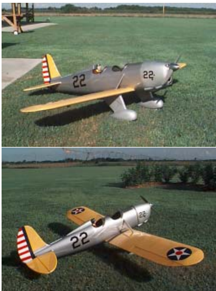
Above, is the latest addition to Bill Bishop's fleet. This is a Ryan STA-M scale military ARF from Great Planes. It has an 82 inch wingspan and weighs around 12 to 14 pounds. All the covering is MonoKote, and Bill said it needed a little ironing to make it look like this. (What looks like wrinkles in the bottom picture are reflections as you can see by comparing it to the top picture.) This beauty is powered by an OS 1.08 engine and Bill says it flies very, very well.
