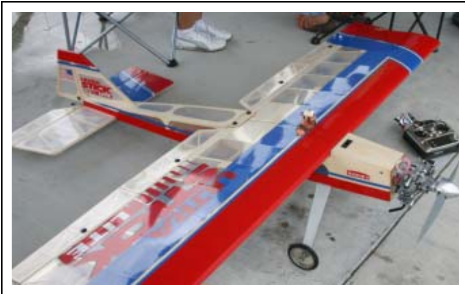
Above, Scott Henry's new Ultra Stick that won the climb and glide contest. Note the 4 stroke 2 cylinder engine on the front.
