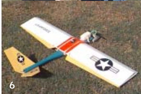
Photo 1: Brand new Edge 540, fully decked out with Sky High graphics. Photo 2, shows the builder, Mike Laughlin with the model and Photo 3, shows the underside treatment. Photo 4: Chief Instructor, Bill Bishop on the buddy box with Junior Member Alvaro Prieto. Photo 5, shows Alvaro with his trainer. Photos 6 & 7 shows Nick Capone's latest project. The fuselage is made from a Wiffle Ball bat and the surfaces are made from corrugated plastic. It flies really well on a .26 engine. Photo 8: Charlie Driggers shows off his new Bi-Plane. He cut down the wings until it would just fit inside the bed of his pickup. Photo 9: Charlie's delta wing plane was built from plans and is fast. Photo 10, shows Bob Cox with his big 4-Star. He says it's a fun airplane to fly. Photo 11: Chip Cipolato's Extra 300 that had an accident not long ago. Chip failed to plug in his aileron servos. He was able to fly with rudder and elevator, but was unable to land it. Photo 12, show the replacement plane he's using until the Extra is repaired.
