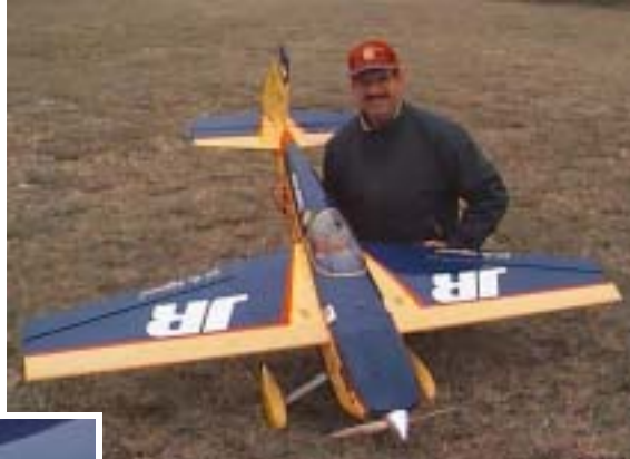
Mike Laughlin and his new Hanger 9 Edge 540 ARF. The plane has a 78 inch wing span, weighs 12.5 pounds and is powered by a OS 1.60. Graphics are by Mike's own Sky High Graphics and the hardware is from Aero Protect. Left, is the very scale cockpit including a VoltWatch so the on-board batteries can be visually monitored. Mike says the plane flies very well and has unlimited vertical.
