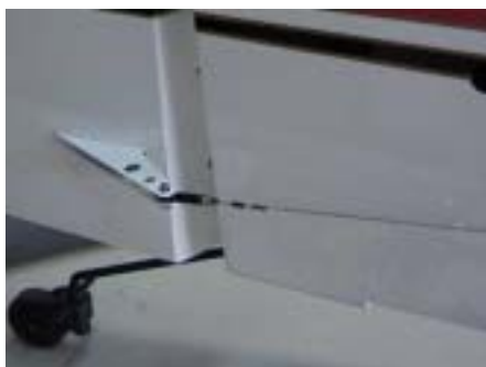
Matching 5 inch rudder control horn with pull-pull cable.
